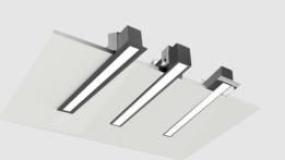
MANUFACTURER Current KIM **PRODUCT** Pursuit - Recessed **PRODUCT TYPE** Ceiling **POWER** 13W-103W VOLTAGE UNV LUMINOUS FLUX 823lm-10578lm ССТ 2700К, 3000К, 3500К, 4000К, 5000К CRI 70, 80, 90 DISTRIBUTION Symmetric, Asymmetric, Wall Graze, Wall Wash **CONTROL** 0-10V (standard) **IP RATING** 66 **IK RATING** 8 **OPERATING TEMPERATURE** -25°C to 40°C LED LIFETIME L70/60,000hrs WARRANTY 5 years MANUFACTURER'S WEBSITE https://www.currentlighting.com/outdoor-lighting/pursuit-recessed/9 109440
