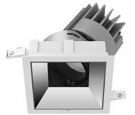
MANUFACTURER Illure PRODUCT Pro Downlight PROSQ125A **PRODUCT TYPE** Ceiling **MOUNTING TYPE** Recessed **POWER** 18W, 25W **VOLTAGE 36V** LUMINOUS FLUX 1300-1800lm сст 3000К, 4000К **CRI** >90 DISTRIBUTION 20°, 40°, 50° **REFLECTOR** Matt Silver, White, Black CONTROL Non-Dim, Phase Dim, 1-10V, DALI **IP RATING 20** SCDM 3 UGR UGR < 16 LED LIFETIME L80 B10/50,000hr WARRANTY 5 Years MANUFACTURER'S WEBSITE https://illurelighting.com.au/product/ildsq-pro125a/
