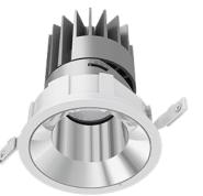
MANUFACTURER Illure PRODUCT Pro Downlight PRO100F **PRODUCT TYPE** Ceiling **MOUNTING TYPE** Recessed **POWER** 13W, 18W **VOLTAGE 36V** LUMINOUS FLUX 900-1300lm сст 3000К, 4000К **CRI** >90 **DISTRIBUTION 28°, 35°, 50° REFLECTOR** Matt Silver, White, Black CONTROL Non-Dim, Phase Dim, 1-10V, DALI **IP RATING 20** SCDM 3 UGR UGR < 16 LED LIFETIME L80 B10/50,000hr WARRANTY 5 Years MANUFACTURER'S WEBSITE https://illurelighting.com.au/product/ild-pro100-f/
