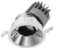
MANUFACTURER Illure PRODUCT Pro Downlight PRO100A **PRODUCT TYPE** Ceiling **MOUNTING TYPE** Recessed **POWER** 13W, 18W **VOLTAGE 36V** LUMINOUS FLUX 850-1200lm сст 3000К, 4000К **CRI** >90 DISTRIBUTION 20°, 40°, 50° **REFLECTOR** Matt Silver, White, Black, Specular CONTROL Non-Dim, Phase Dim, 1-10V, DALI **IP RATING 20** SCDM 3 UGR UGR < 16 LED LIFETIME L80 B10/50,000hr WARRANTY 5 Years MANUFACTURER'S WEBSITE https://illurelighting.com.au/product/ild-pro100-a/
