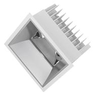
MANUFACTURER Illure PRODUCT Classic Downlight ILDSQ150 **PRODUCT TYPE** Ceiling **MOUNTING TYPE** Recessed **POWER** 18W, 25W VOLTAGE 36V LUMINOUS FLUX 1500-2200lm сст 3000к, 4000к CRI >90 **DISTRIBUTION** 70° **REFLECTOR** Matt Silver, White, Black CONTROL Non-Dim, Phase Dim, 1-10V, DALI **IP RATING** 54 SCDM 3 UGR UGR < 19 LED LIFETIME L80 B10/50,000hr WARRANTY 5 Years MANUFACTURER'S WEBSITE https://illurelighting.com.au/product/ildsq150/
