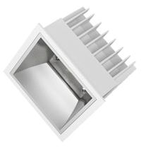
MANUFACTURER Illure PRODUCT Classic Downlight ILDSQ100 **PRODUCT TYPE** Ceiling **MOUNTING TYPE** Recessed **POWER** 9W, 13W VOLTAGE 36V LUMINOUS FLUX 800-1200lm сст 3000к, 4000к CRI >90 **DISTRIBUTION 60° REFLECTOR** Matt Silver, White, Black CONTROL Non-Dim, Phase Dim, 1-10V, DALI **IP RATING** 54 SCDM 3 UGR UGR < 19 LED LIFETIME L80 B10/50,000hr WARRANTY 5 Years MANUFACTURER'S WEBSITE https://illurelighting.com.au/product/ildsq100/
