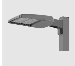
MANUFACTURER Current BEACON **PRODUCT** Beacon Viper Area, Strike **PRODUCT TYPE** Outdoor **POWER** 39W-545W VOLTAGE UNV LUMINOUS FLUX 5500Im-60000Im ССТ 2700К, 3000К, 3500К, 4000К, 5000К CRI 70, 80 DISTRIBUTION Type FR, Type 2, Type 3, Type 4F, Type 4W, Type 5QN, Type 5QW, Type 5QM, Type 5W, Type 5RW, Type C, Type TC **CONTROL** 0-10V (standard) **IP RATING** 65 **OPERATING TEMPERATURE 40°C** WARRANTY 5 years MANUFACTURER'S WEBSITE https://www.currentlighting.com/search?keys=viper
